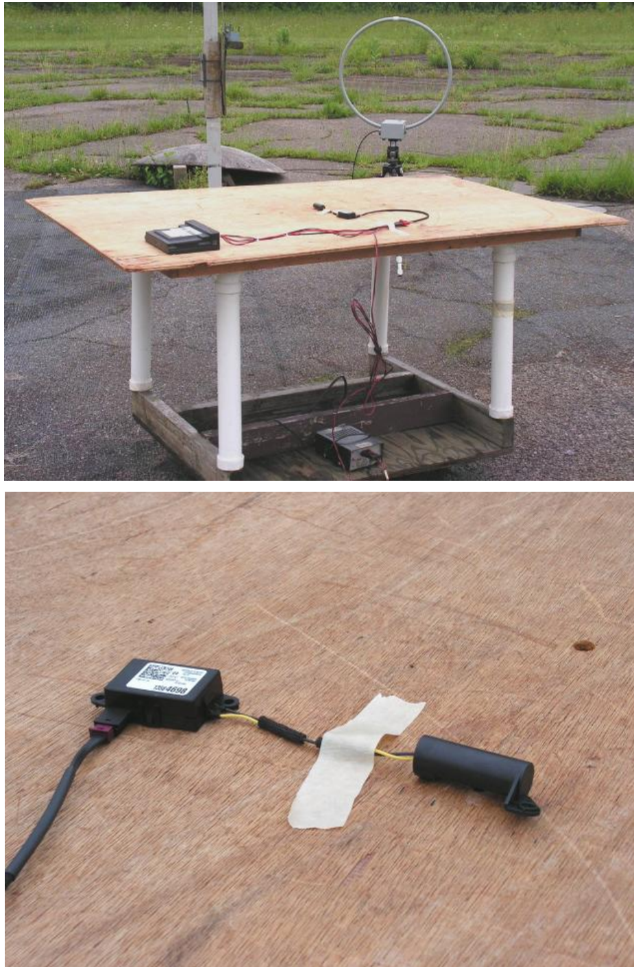
Figure 4: Radiated Emissions Test Setup Photograph(s).
