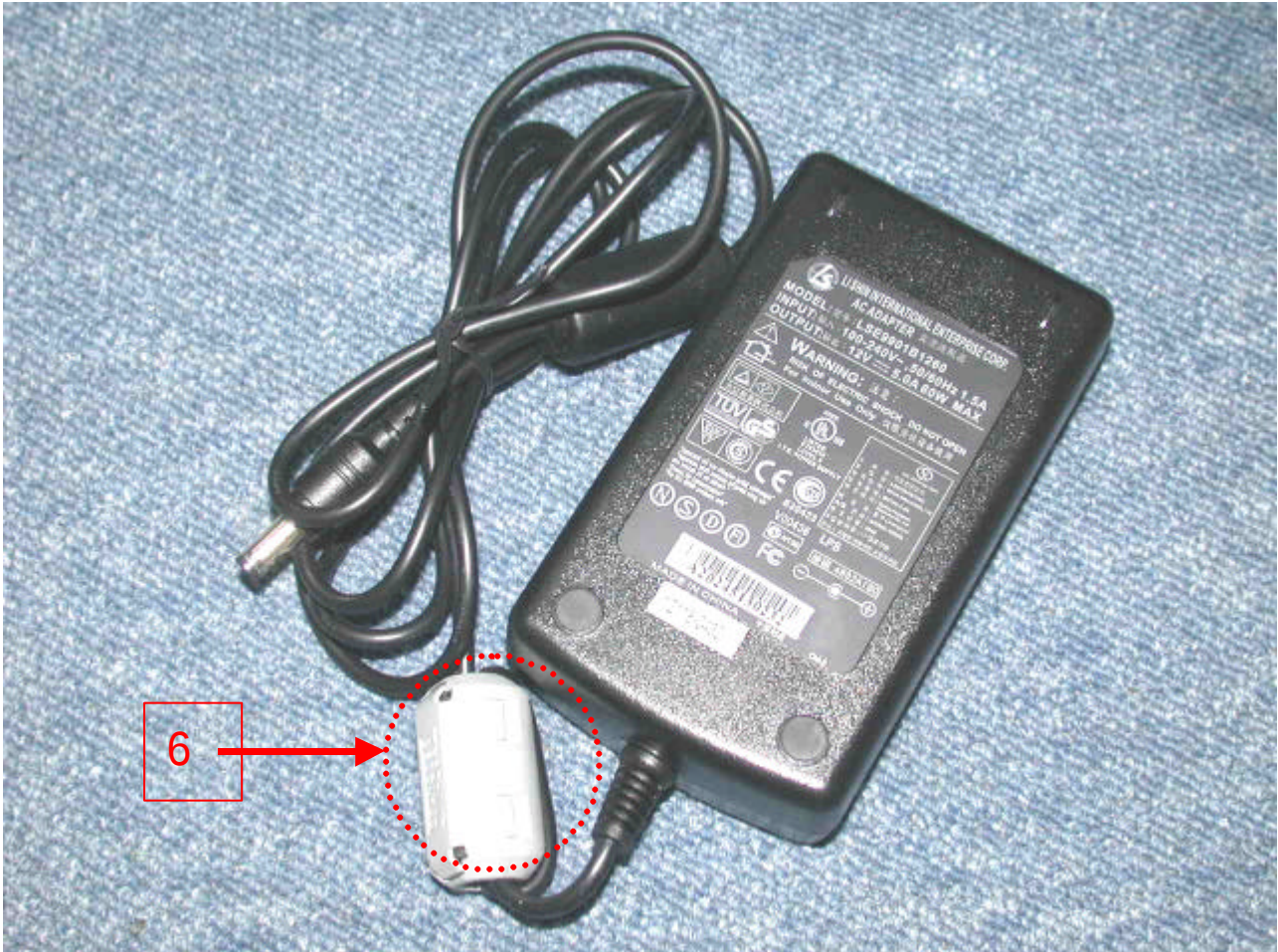
6. Ferrite core (TDK/ZCAT2035-0930) added in DC Power cable
