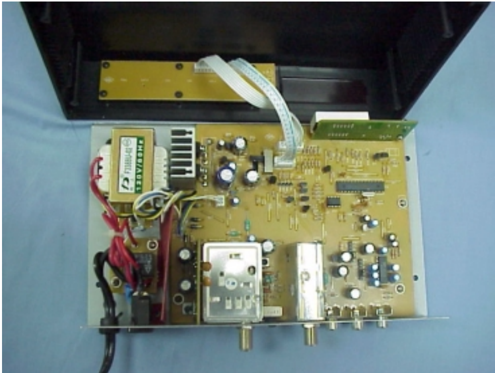
Figure 2 Remote Control Cable Converter (M/N: F3388U) MAIN BOARD (COMPONENT SIDE)
