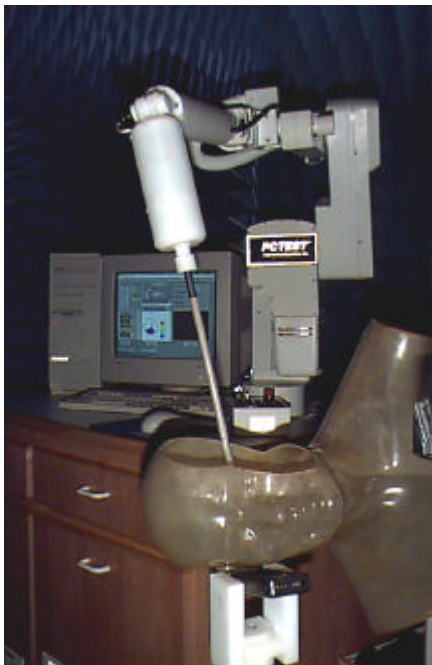
Figure 5. Photograph of the Probe and the Phantom
