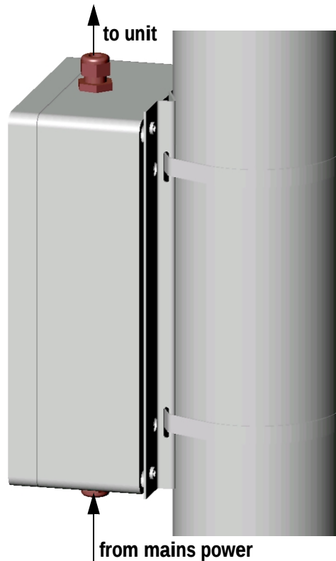
figure 9. power supply installation - pole
