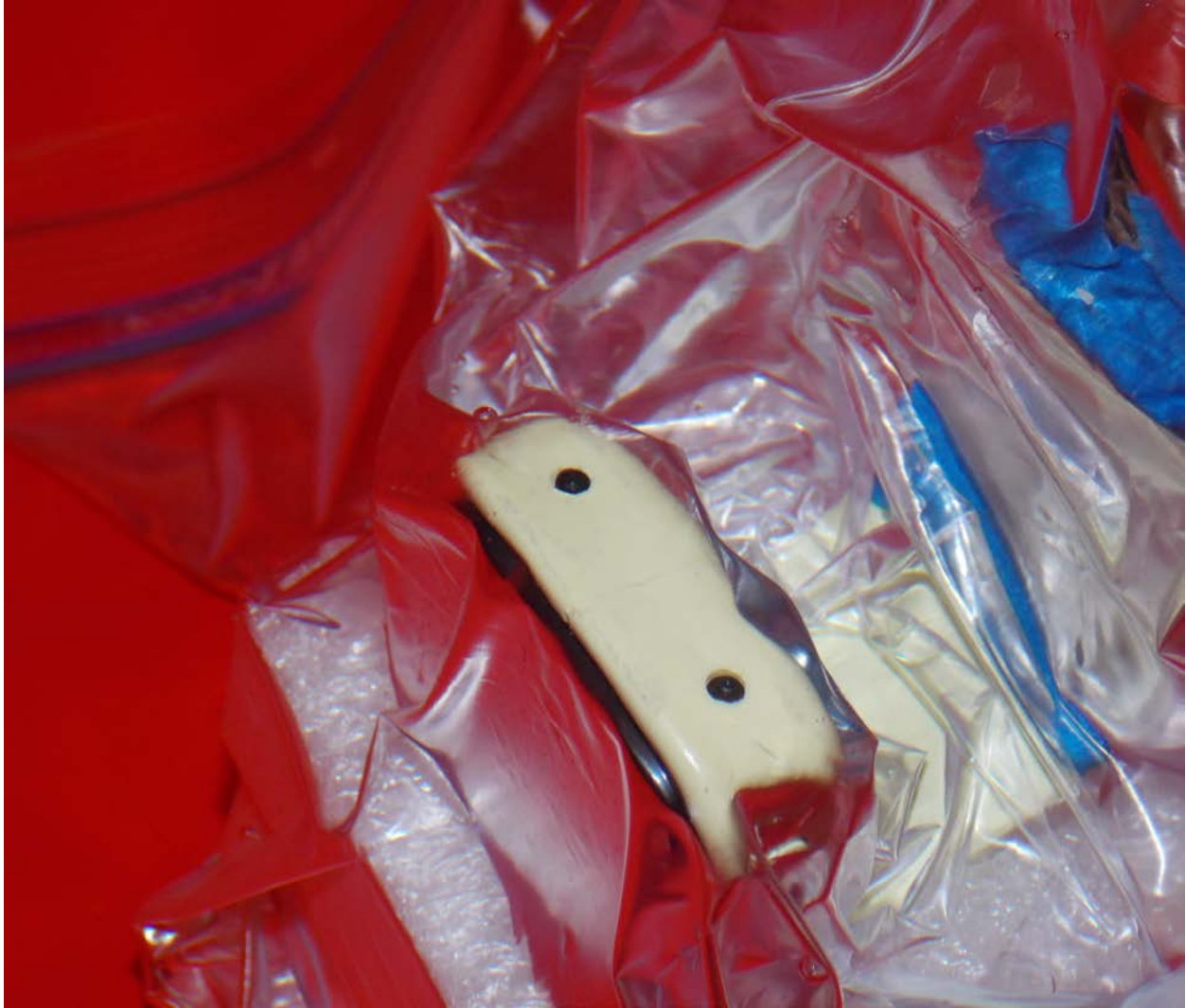
Device Set in Tissue For Extremity Testing
