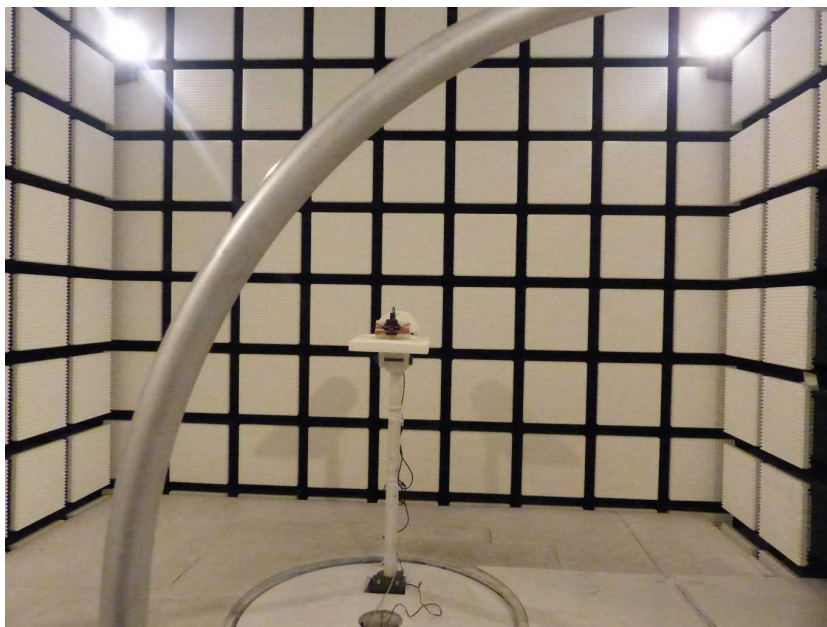
Photo 4: Radiated measurements fully anechoic chamber
