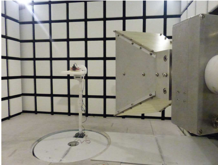
Photo 3: Radiated measurements fully anechoic chamber
