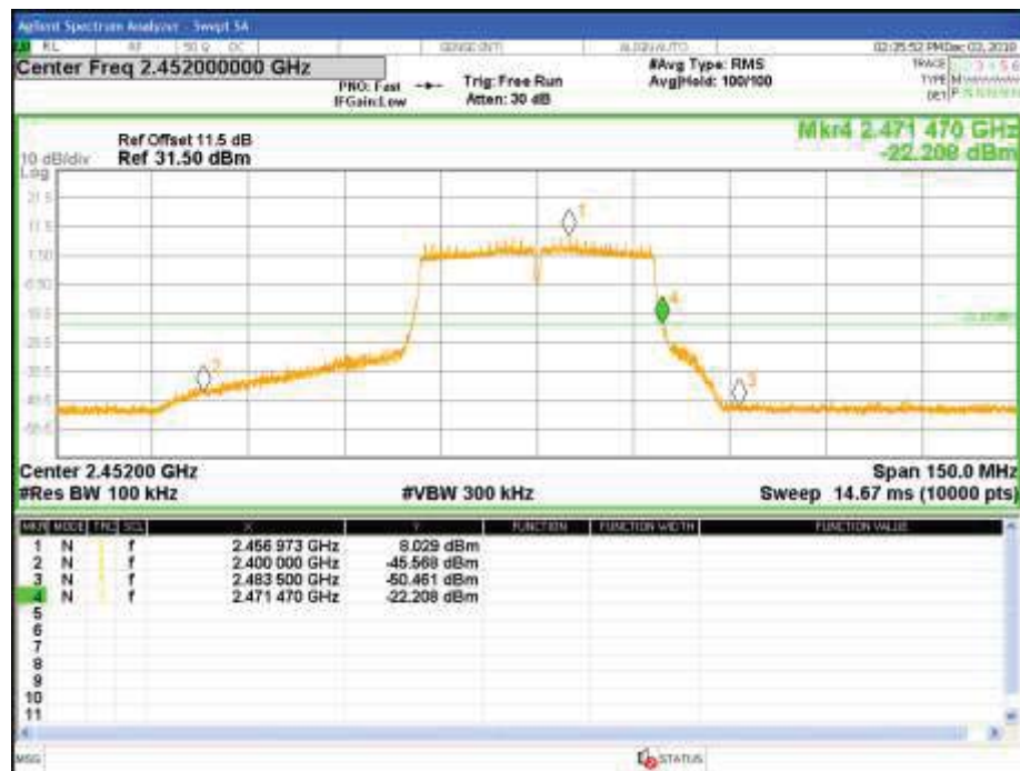
Figure 209: Measured Bandedge at 2483.5MHz-2452MHz-HT40-4x4-Ch2
