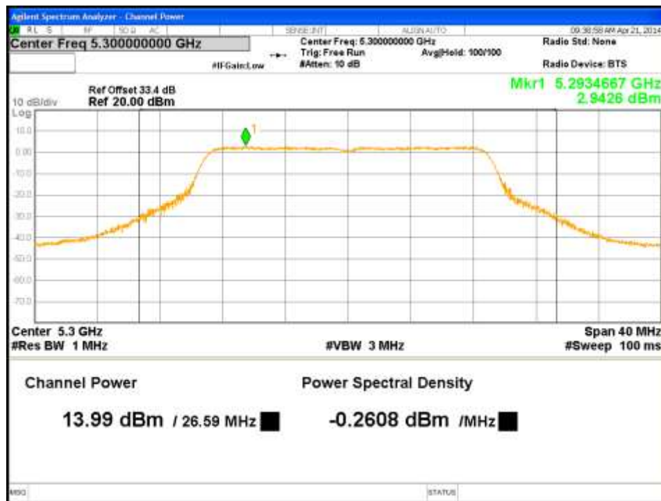
Figure 39: Maximum Conducted Output Power-5300MHz-VHT20-MCS0-Ch2
