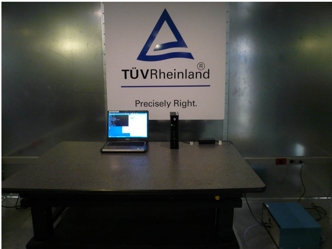
Figure 13: AC Conducted Emission Test Setup (Front View)
