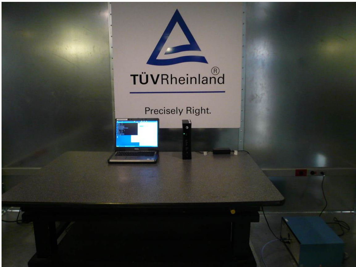
Figure 13: AC Conducted Emission Test Setup (Front View)
