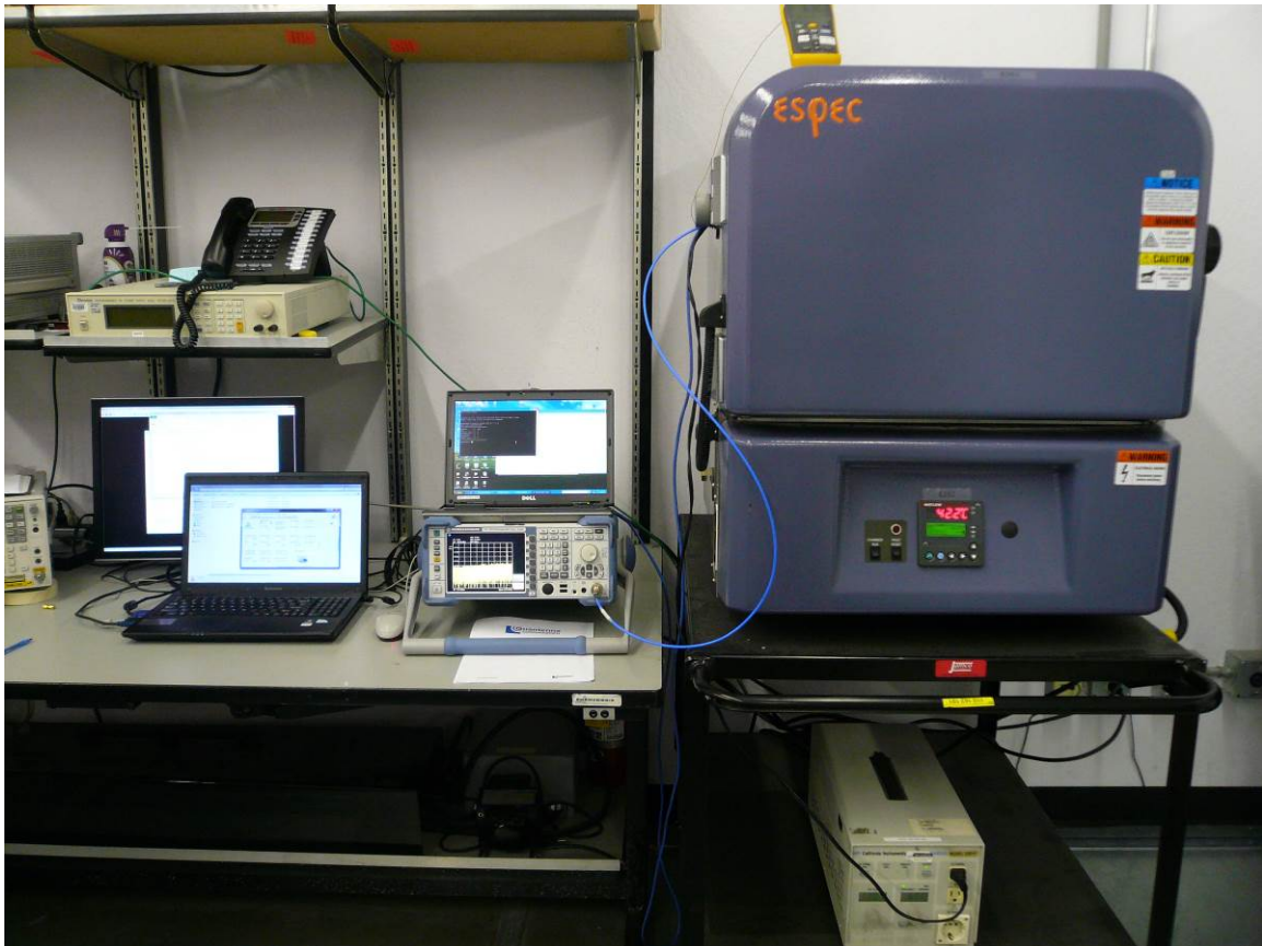
Figure 12: Extreme Condition Test Setup – Outside Thermo Chamber
