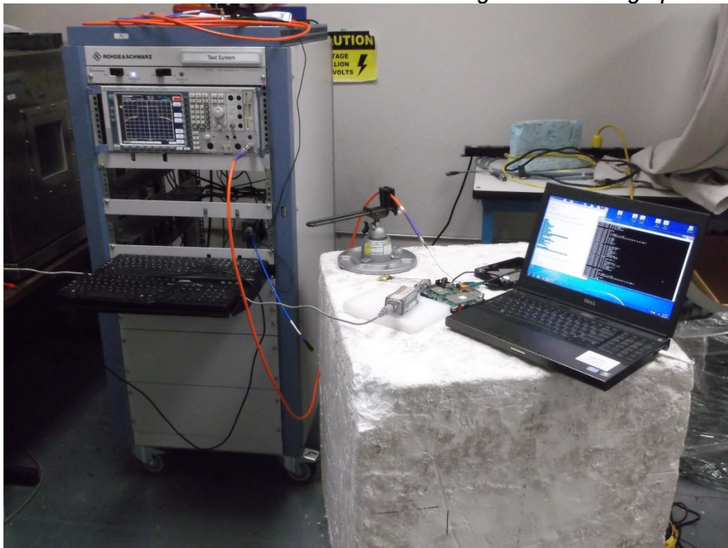
Antenna Conducted Emissions Test Configuration Photographs
