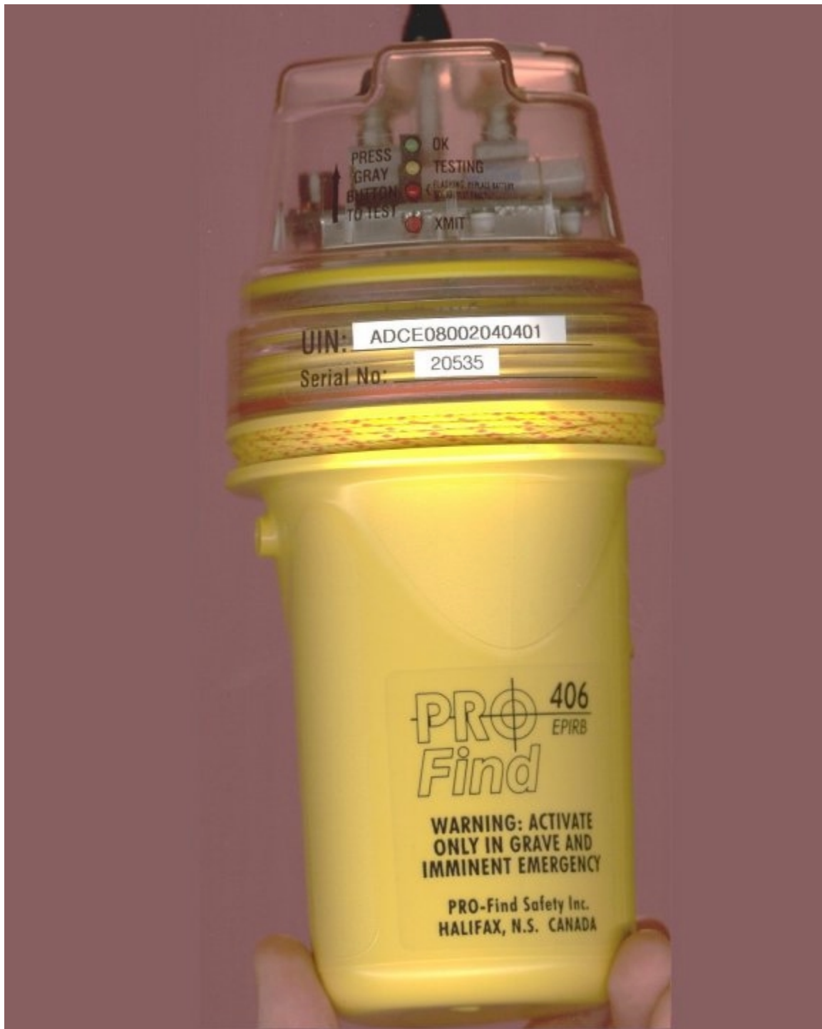
Photograph 1. Close up of EPIRB
