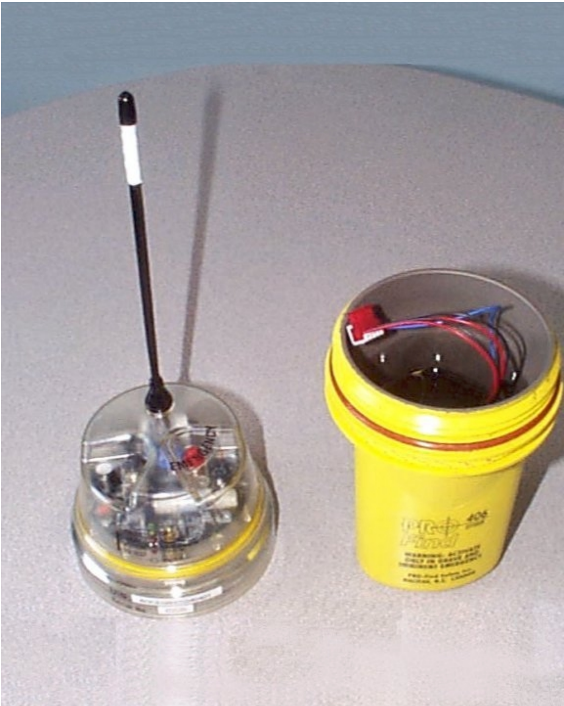
Photograph 4. EPIRB and Battery
