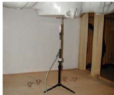
Figure 12.1 Dipole Validation Test Setup
