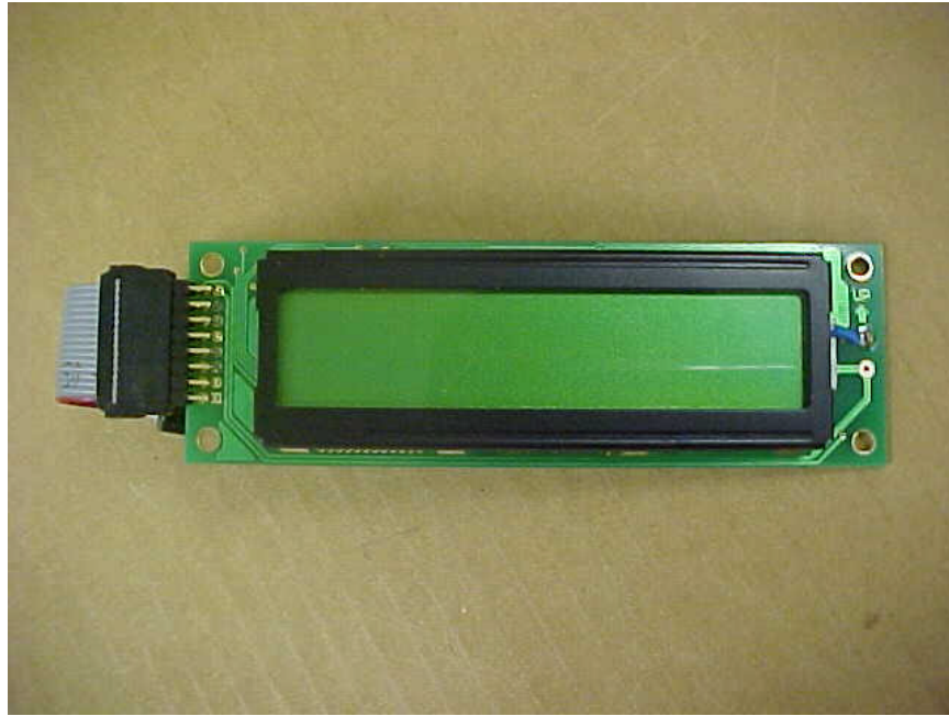
Close look at the Front Liquid Crystal Display Model NDM20216L-1-L30S
