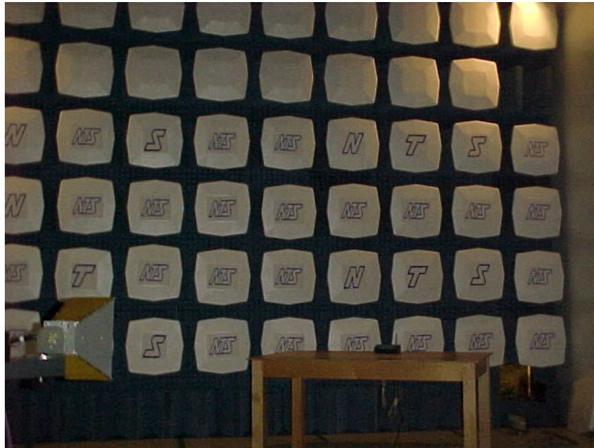
Radiated Emissions (FCC Chamber), Front of EUT 1-10GHz
