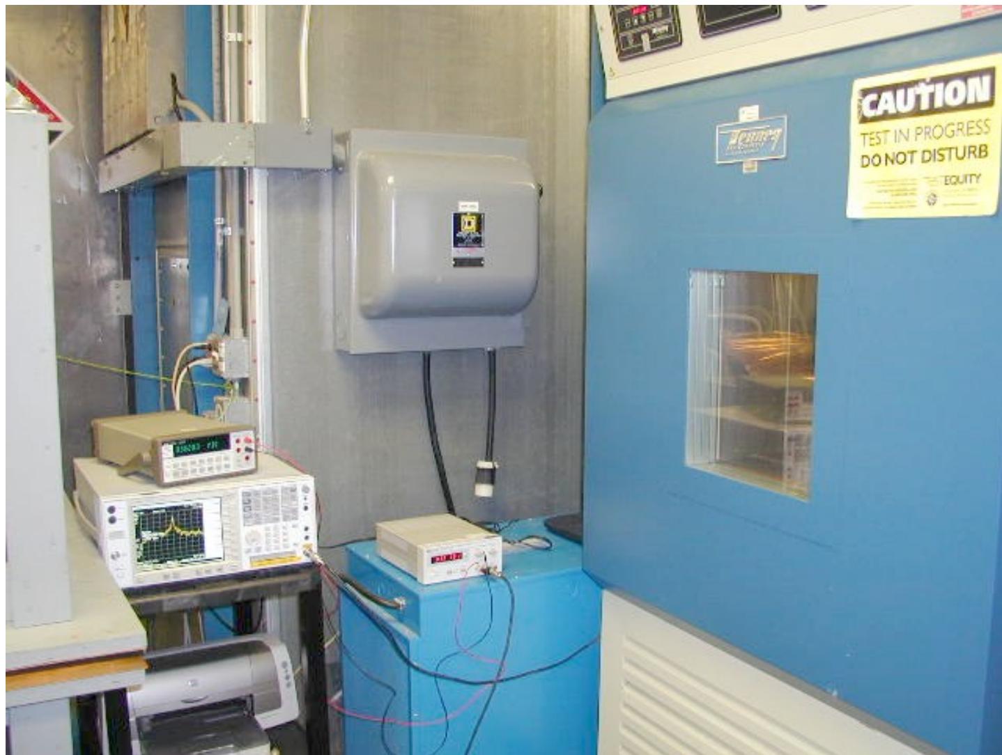
Photograph of Test Setup: Frequency Stability
