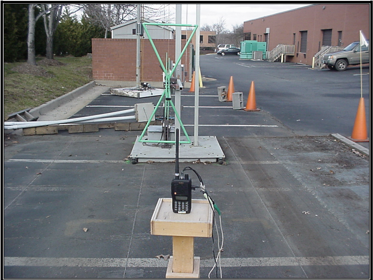
Photograph 3: Radiated Emissions Test Configuration (Front View)
