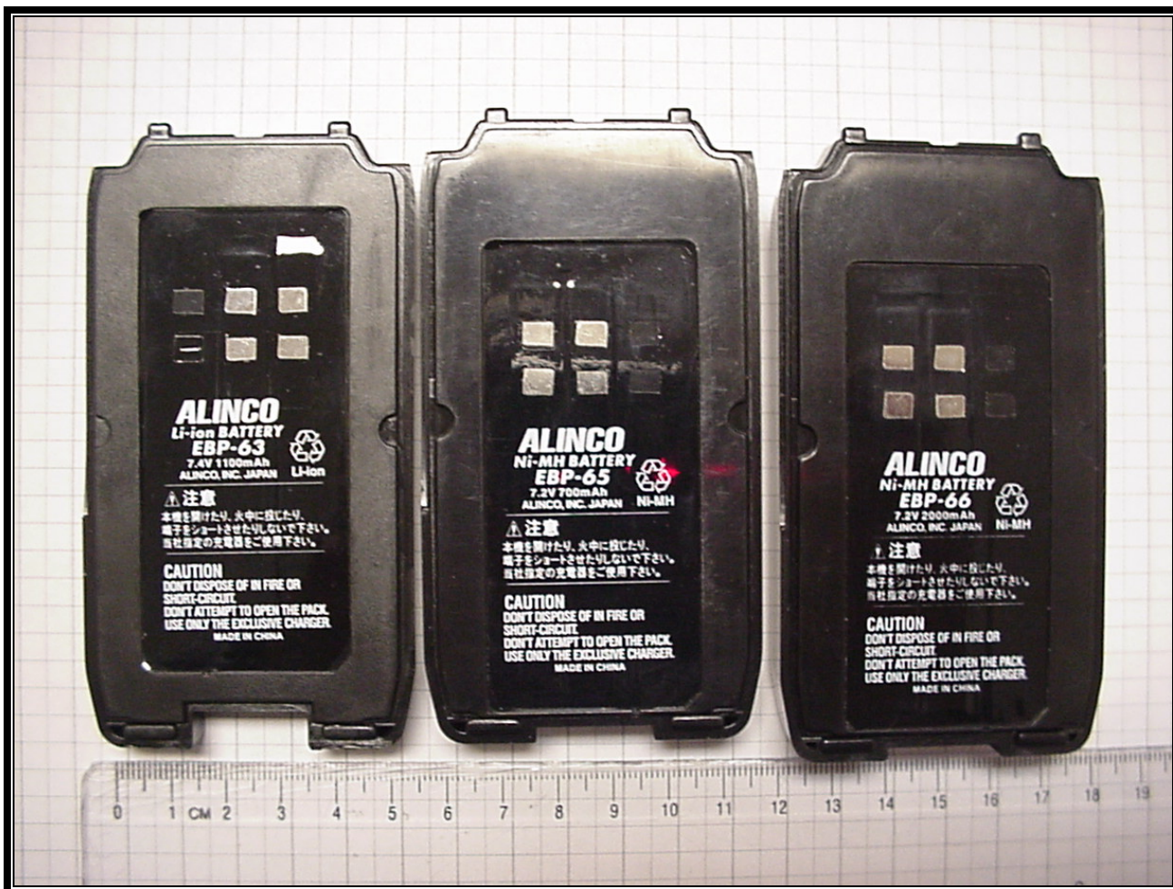
Photograph 15: EBP-63, EBP-65, EBP-66 Battery Labels
