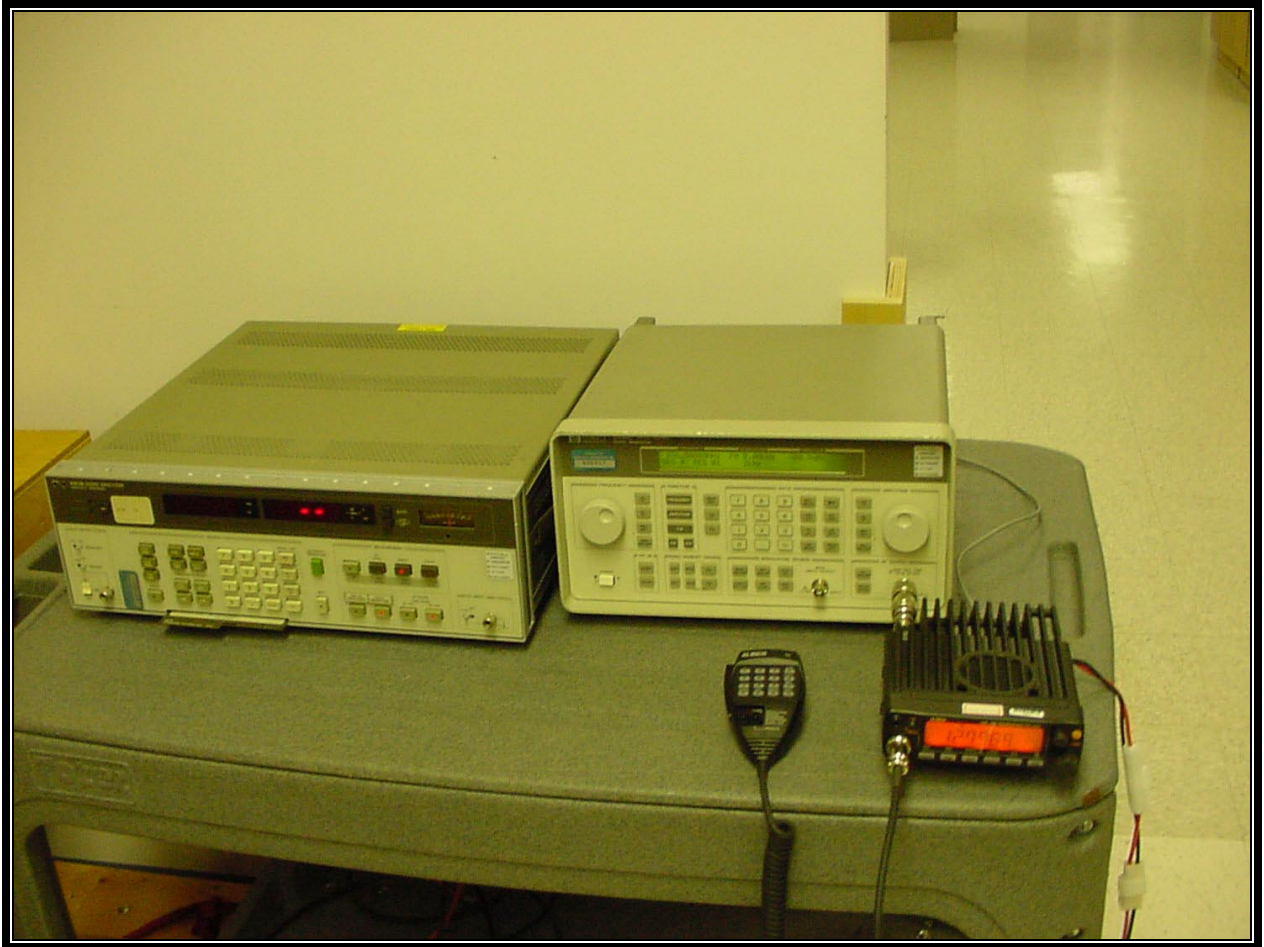
PHOTOGRAPH 4: 38 DB REJECTION TEST CONFIGURATION
