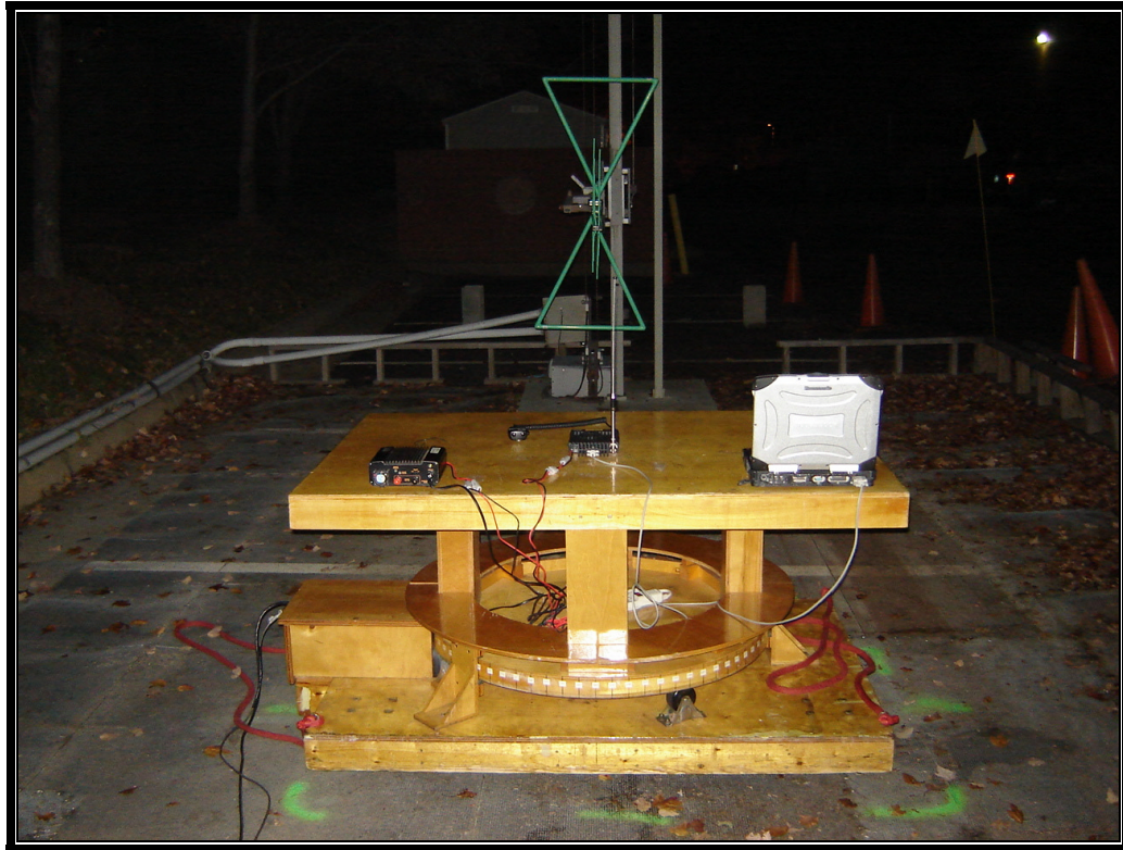
Photograph 4: Radiated Emissions Test Configuration (Rear View)
