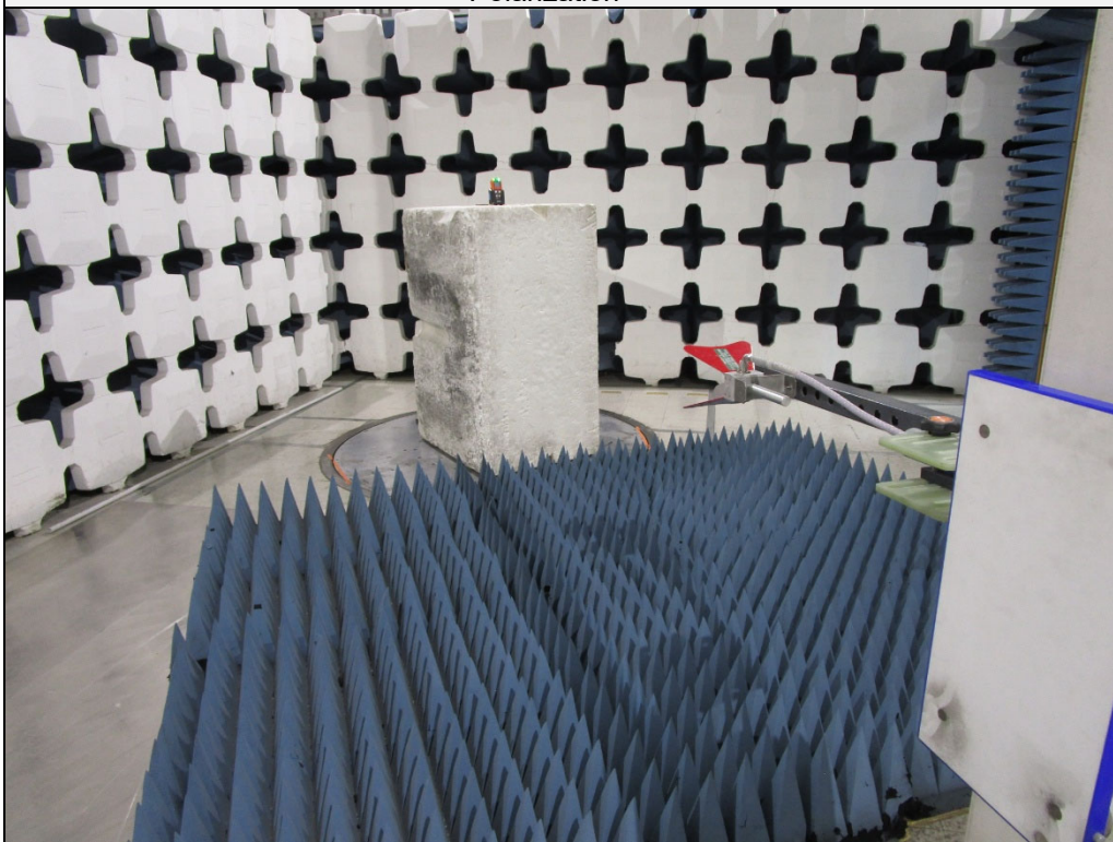
Test Setup for Radiated Spurious Emissions: 1GHz to 18GHz, Vertical Polarization
