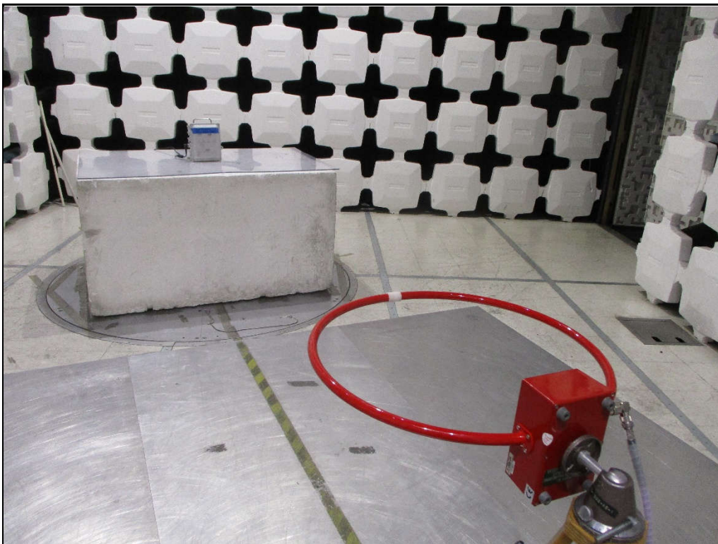
Test Setup for Spurious Radiated Emissions, 10-30MHz – Antenna Polarization Horizontal
