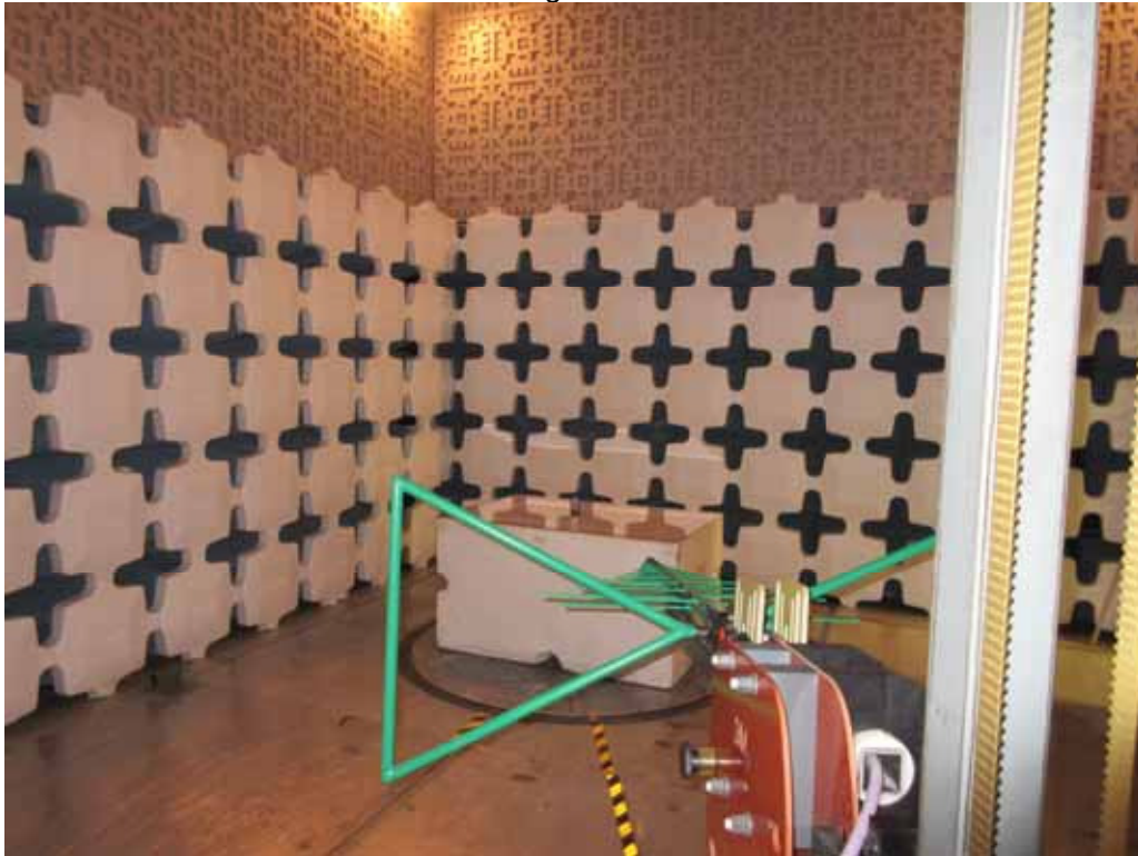
Test Setup for Radiated Emissions above 30MHz – Horizontal Polarization
