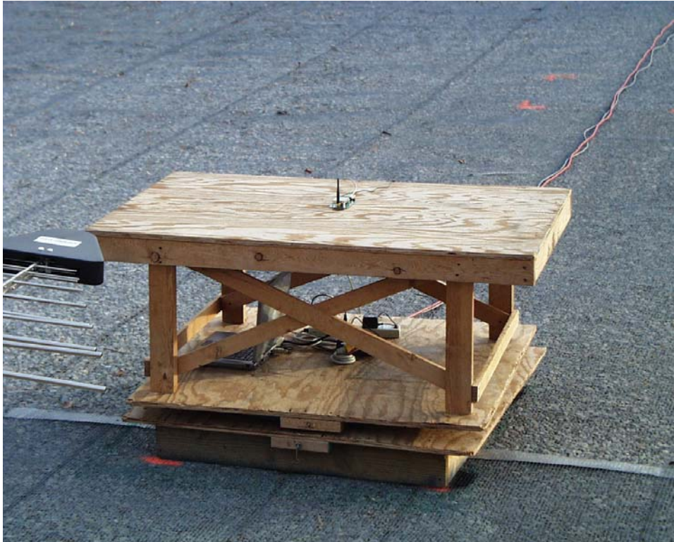
Radiated Emissions Test setup photographs with \frac{1}{4} wave stub antenna. (Part number ANT-915DEV)
