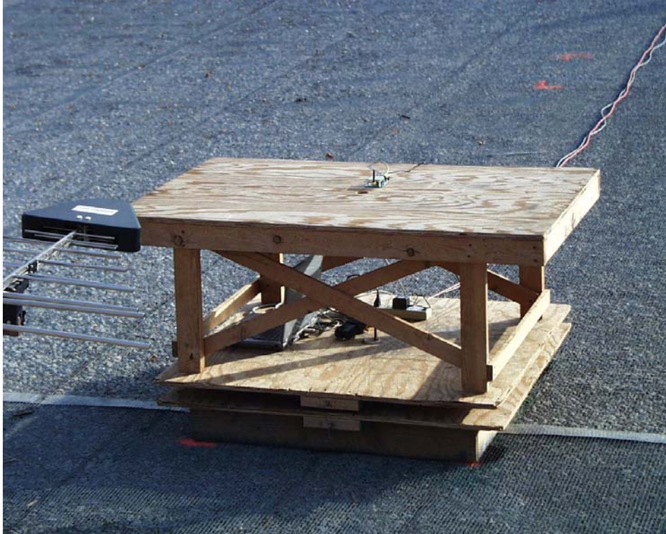
Radiated Emissions Test setup photographs with short \frac{1}{4} wave stub antenna. (Part Number ANT-915CW)
