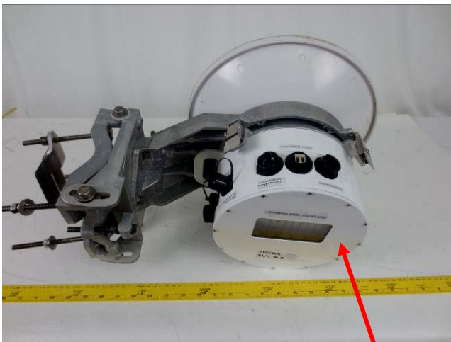
EUT with 1 ft., 45 dBi Antenna
