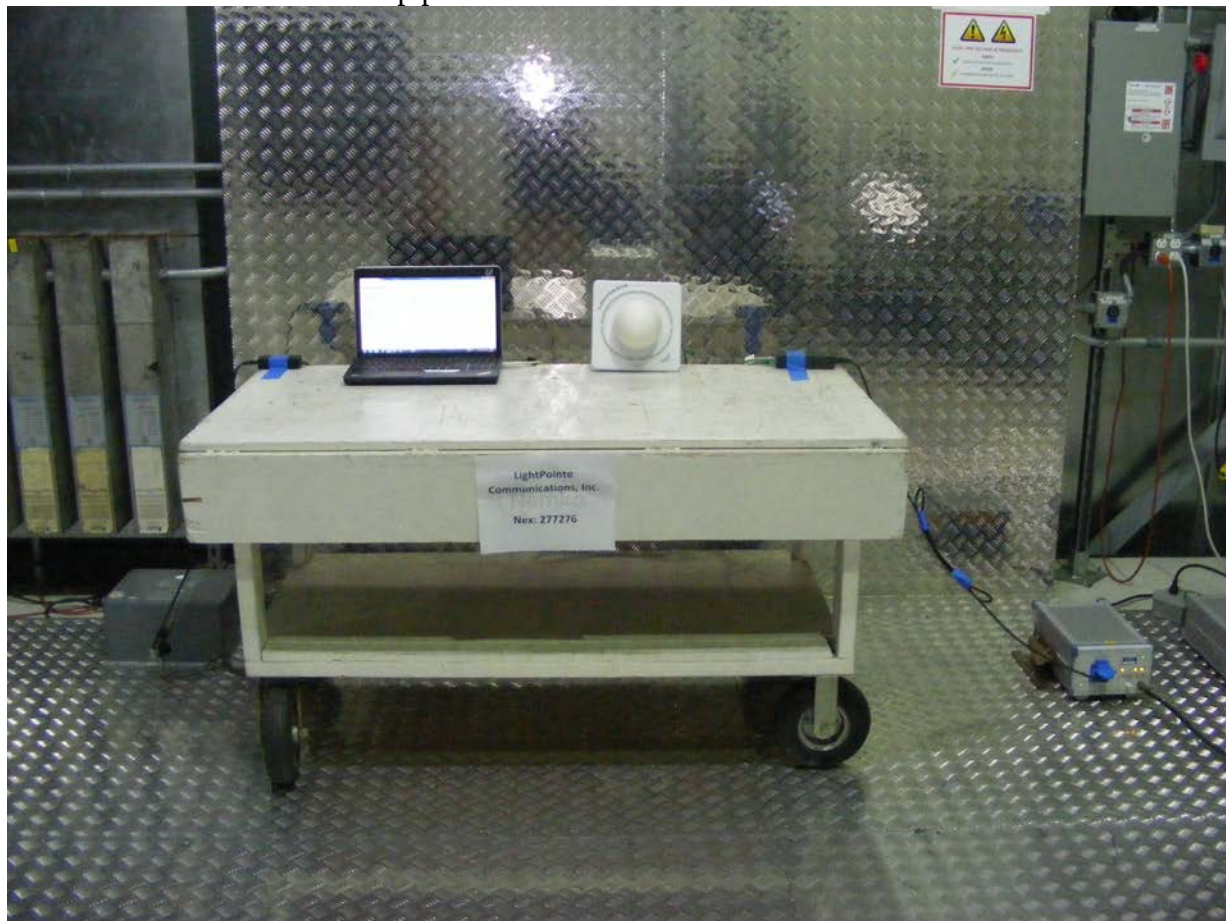
Conducted Emissions test setup photo
