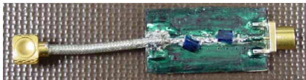
Low Pass Filter Assembly (Top Side)
