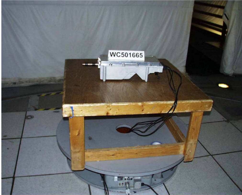
Test-setup photo(s): Radiated emission 30 MHz - 26000 MHz
