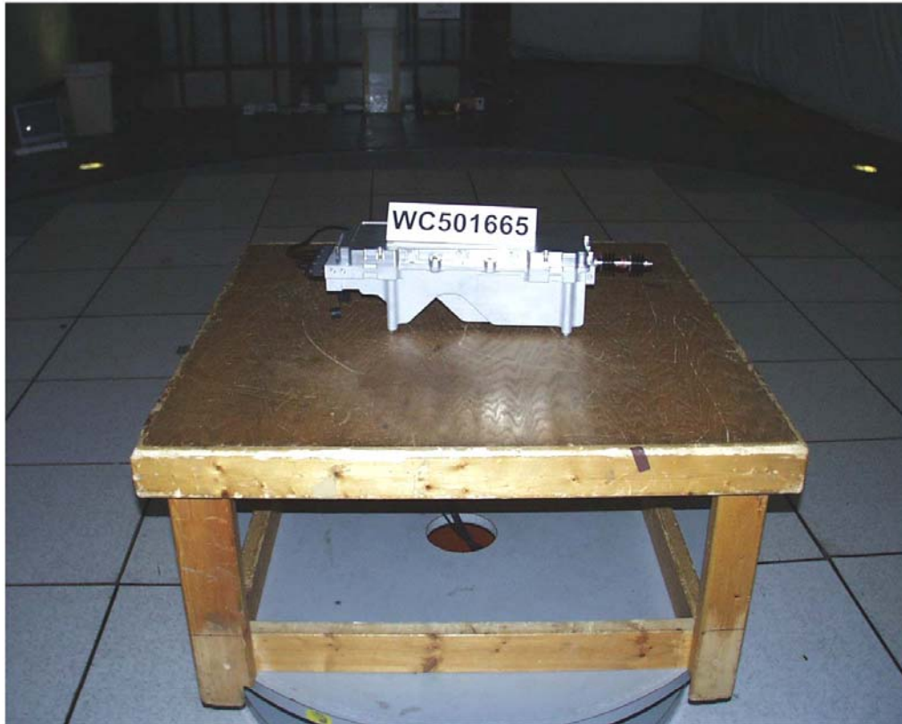
Test-setup photo(s): Radiated emission 30 MHz - 26000 MHz
