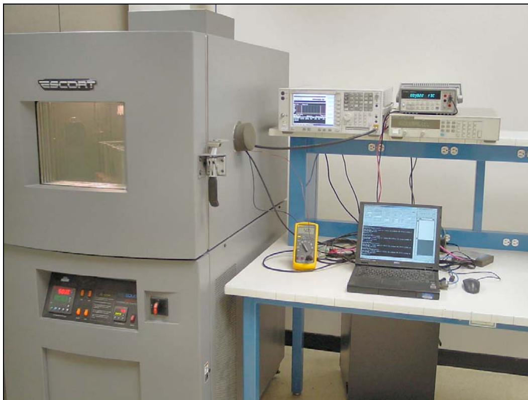
Frequency Stability Test Setup
