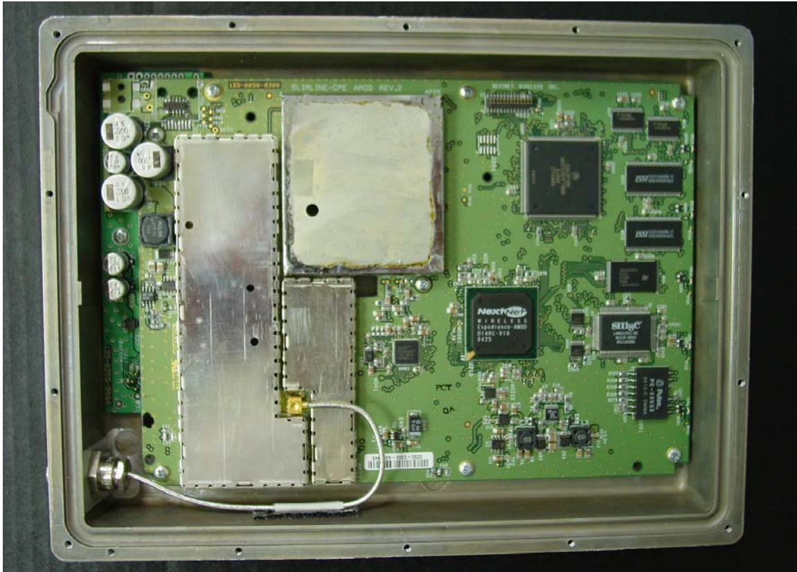
Interface and main board in casting with shields
