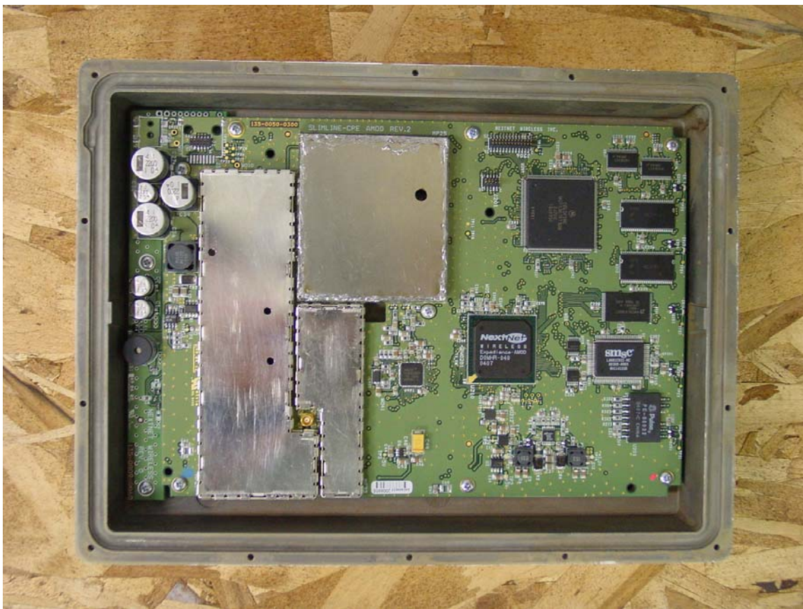
Interface and main board in casting with shields
