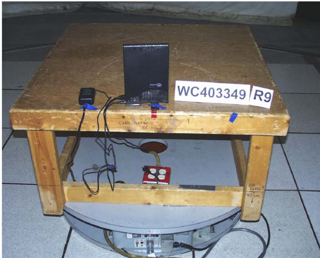
Test-setup photo(s): Radiated emission 30 MHz - 12500 MHz
