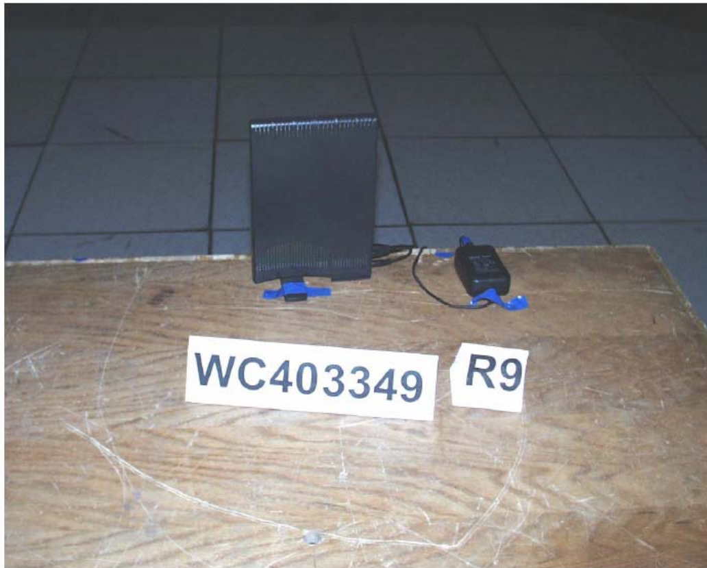
Test-setup photo(s): Radiated emission 30 MHz - 12500 MHz
