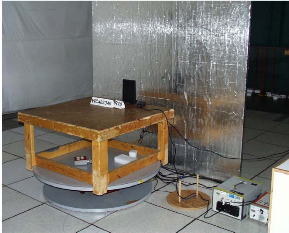
Test-setup photo(s): Conducted emission 10/150 kHz - 30 MHz
