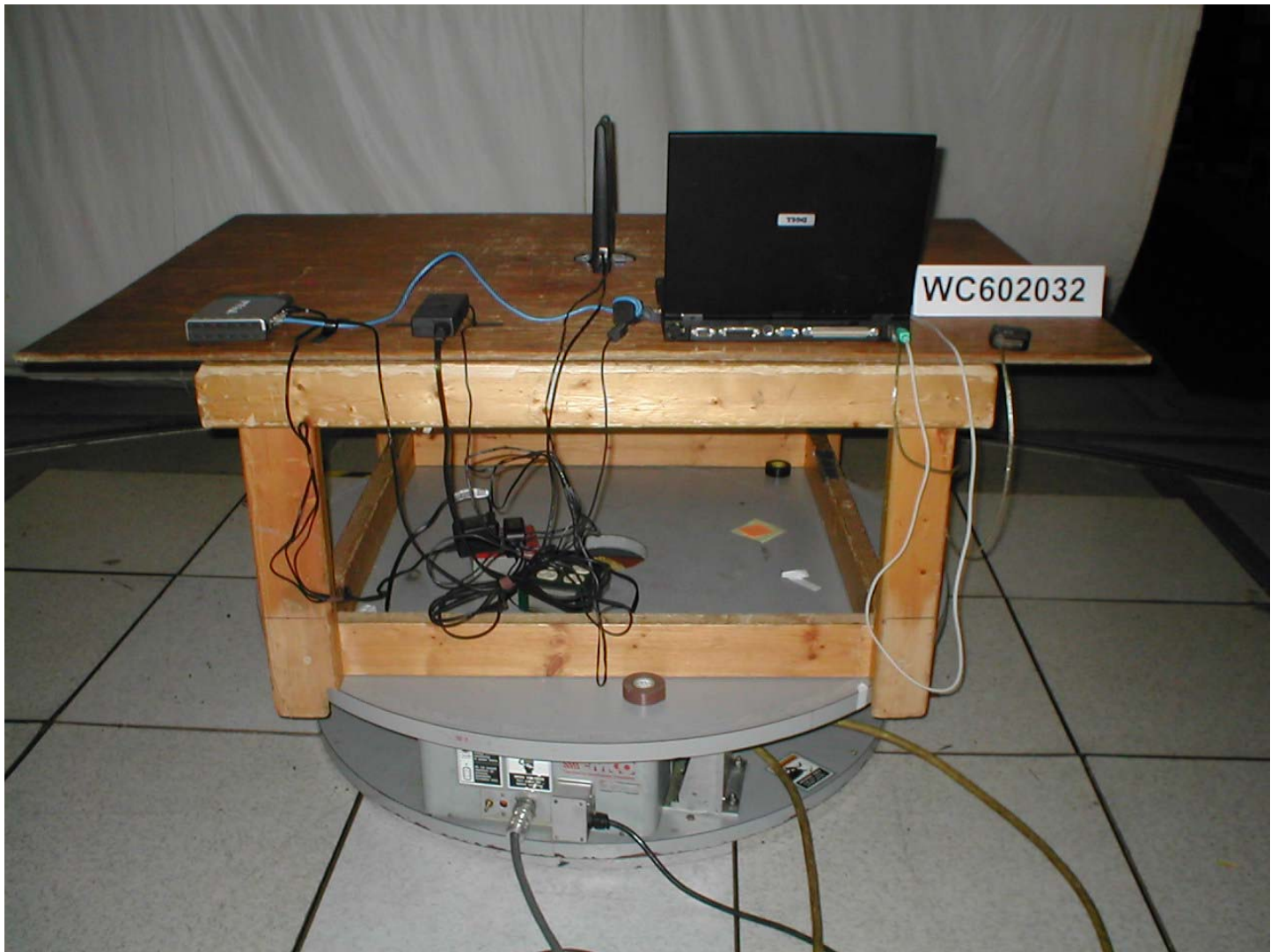
Test setup photo, radiated emissions Testing done under test report number WC602032
