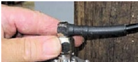
Figure 10: Connecting Antenna RF Cable
