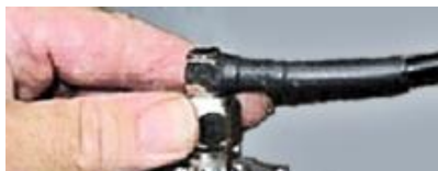
Figure 53: Connecting Antenna RF Cable
