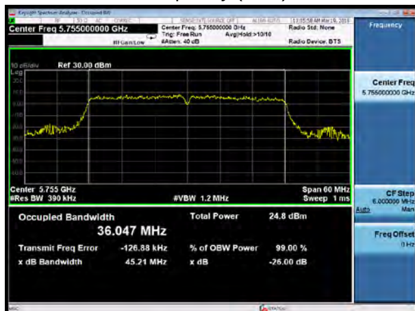
U-NII-3, 802.11ac VHT40 Carrier frequency (MHz): 5755
