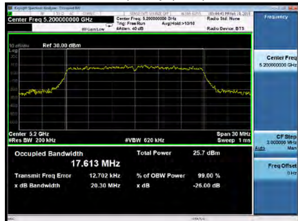
U-NII-1, 802.11ac VHT20 Carrier frequency (MHz): 5240
