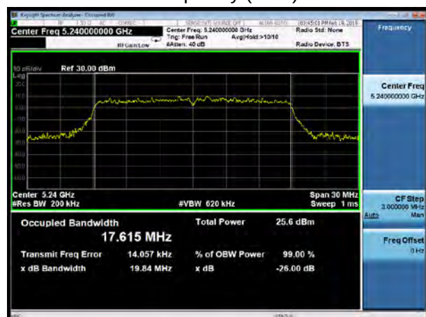
U-NII-1, 802.11ac VHT20 Carrier frequency (MHz): 5240
