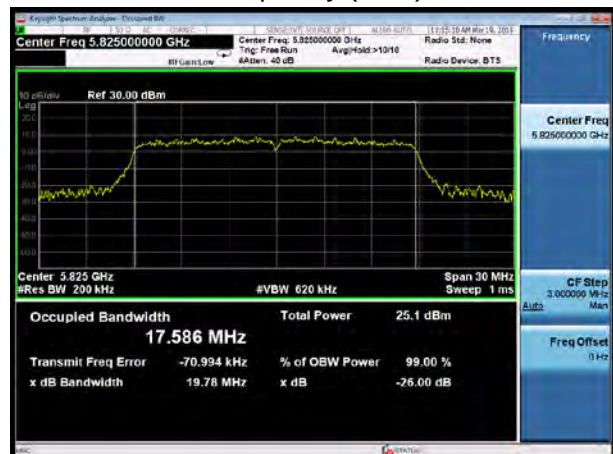
U-NII-3, 802.11ac VHT20 Carrier frequency (MHz): 5825
