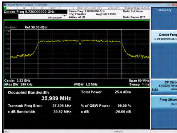
U-NII-1, 802.11ac VHT40 Carrier frequency (MHz): 5190
