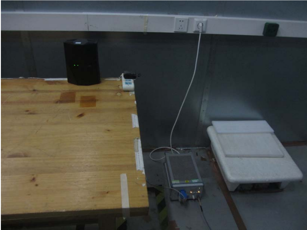
Picture 3 Conducted Emission Test Setup
