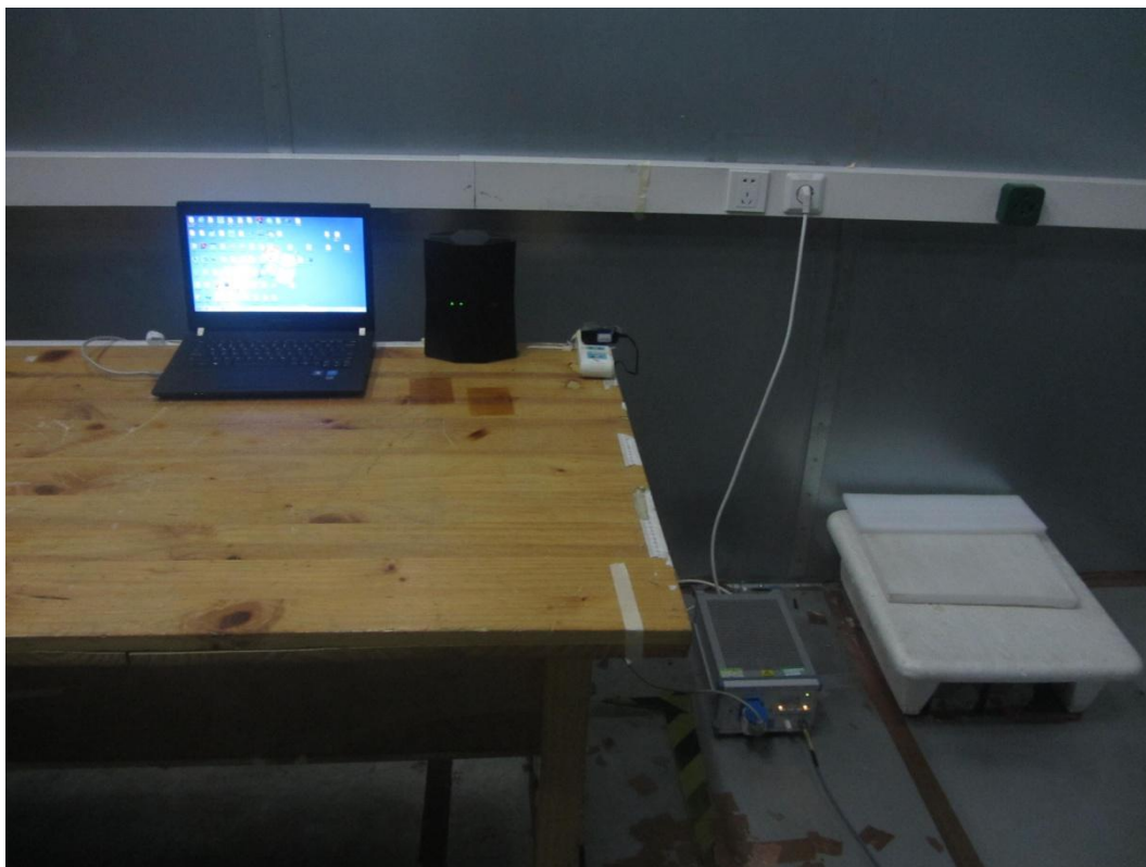
Picture 3 Conducted Emission Test Setup
