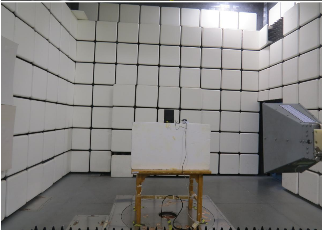
Picture 2 Radiated Spurious Emissions Test setup
