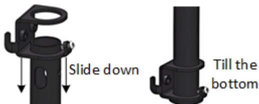
Figure 14: Slide the Hanger onto Pole
