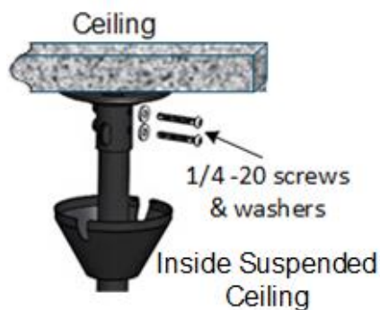
Figure 16: Insert the 2 Screws
