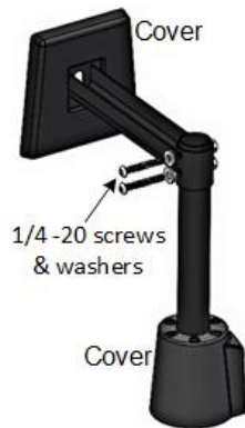
Figure 26: Insert the Screws
