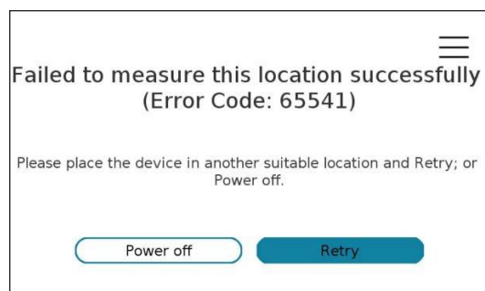
Figure 18 No signal detected
