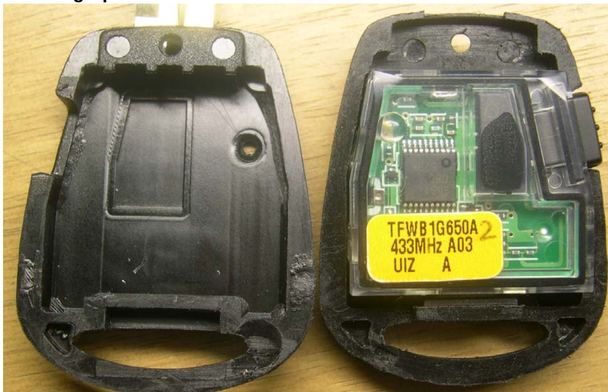
<Photograph 1: Cover removed>
