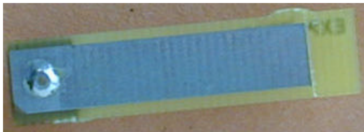
Antenna – Bottom View.
