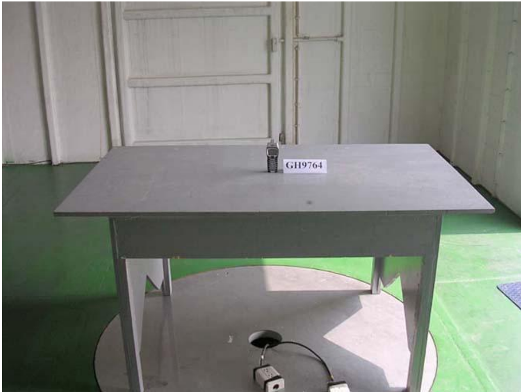
Photo 4: Radiated Emission Test Set-up (Handset)
