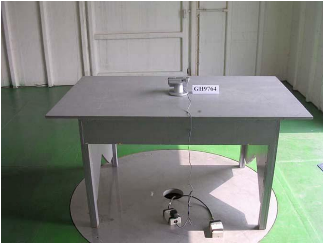
Photo 3: Radiated Emission Test Set-up (Base)
