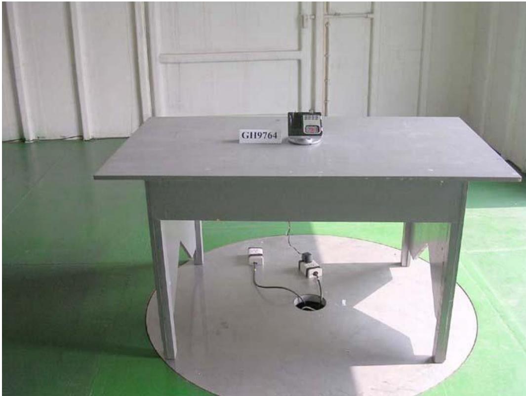
Photo 1: Radiated Emission Test Set-up (Base)
