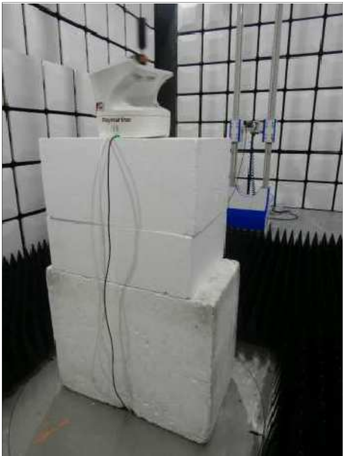
Figure 77 - Test Setup - 18 GHz to 40 GHz
