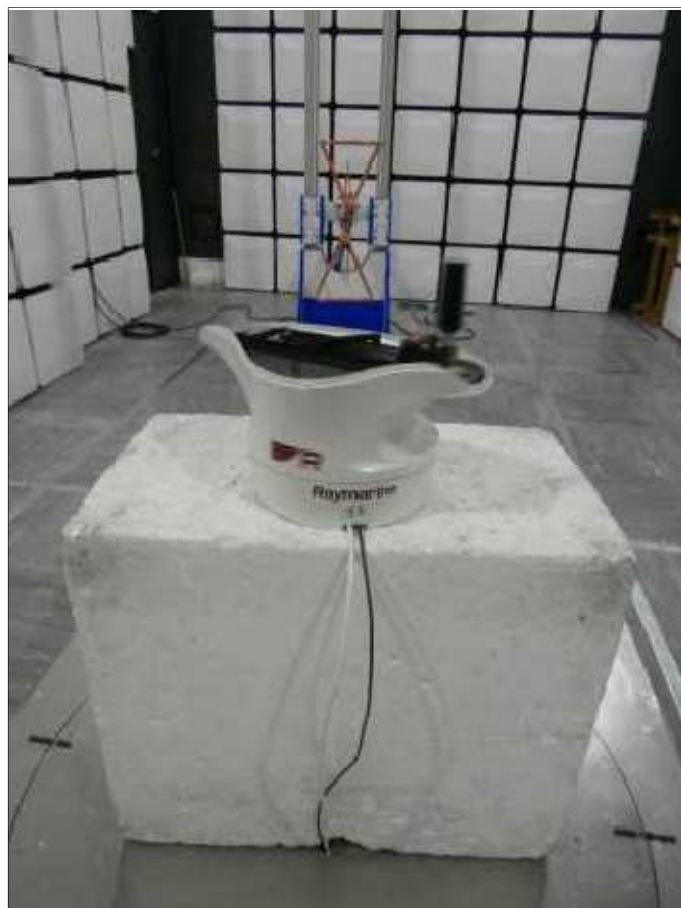
Figure 75 - Test Setup - 30 MHz to 1 GHz
