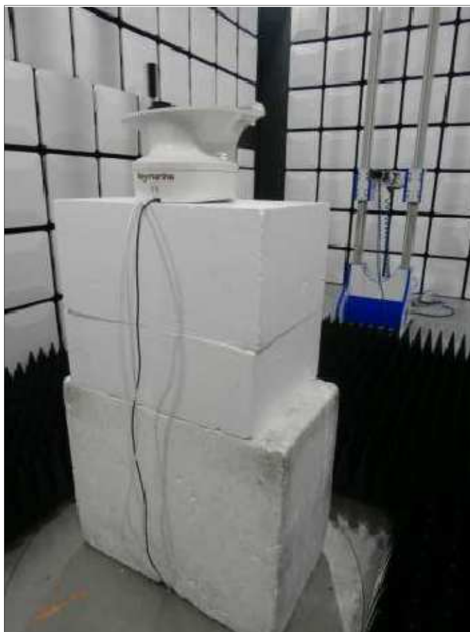
Figure 76 - Test Setup - 1 GHz to 18 GHz
