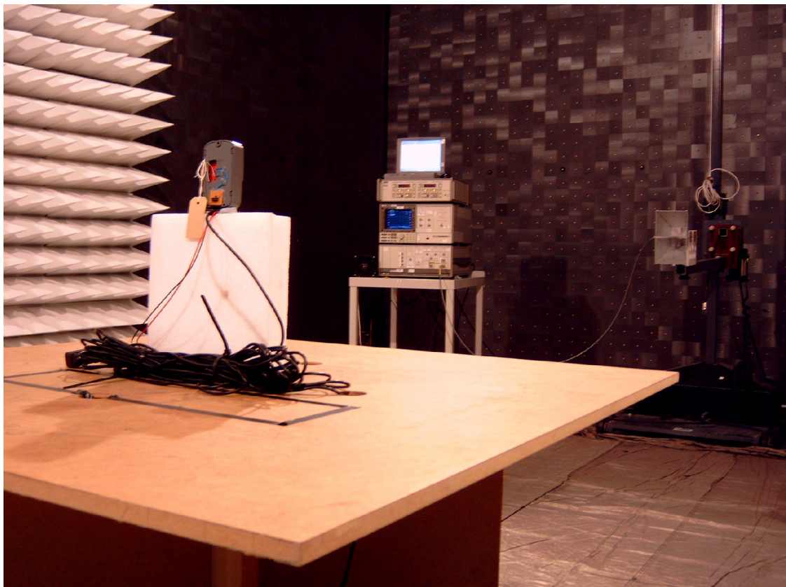
Figure 3 Set up in chamber for 2GHz – 7GHz measurements at 3m.
