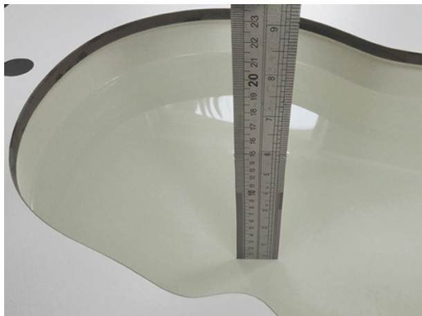
Liquid depth in the head phantom (2450MHz)
