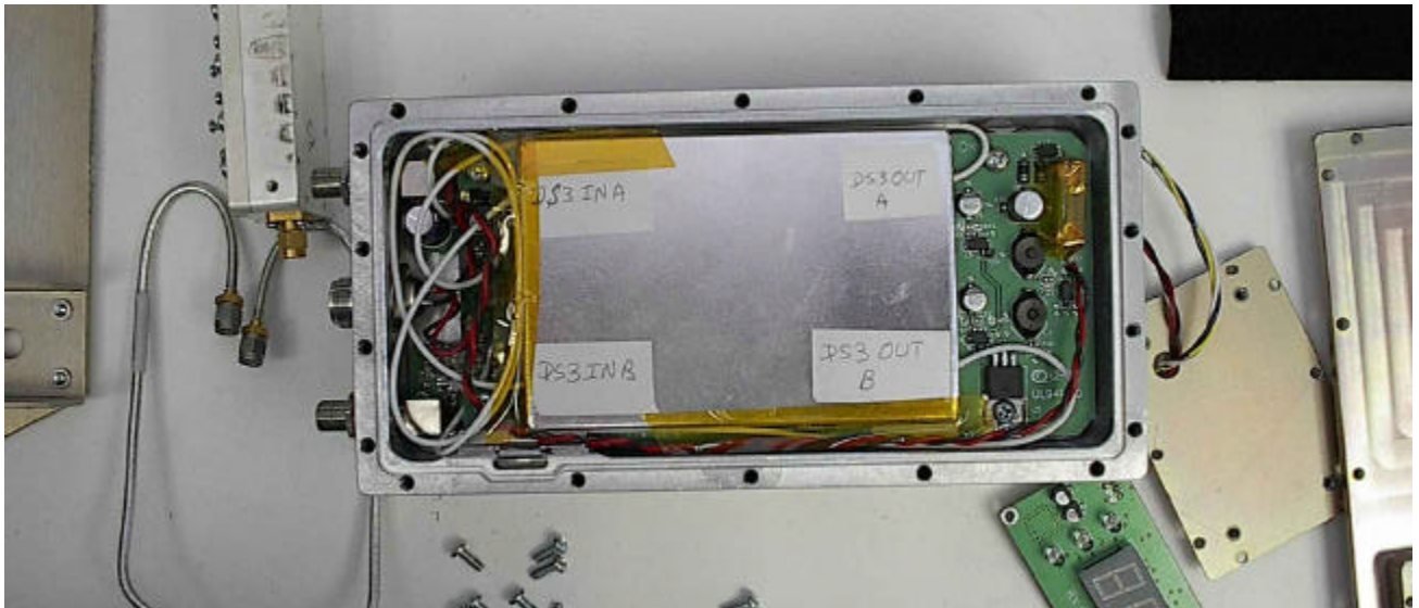
Digital Section – Assembly Top View
