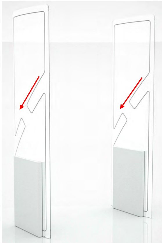
Fig. 7 Conductors shape have to have same direction
