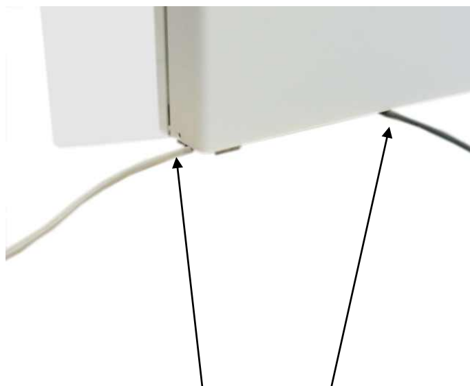
Fig. 7 Cable routing at the antenna sides
