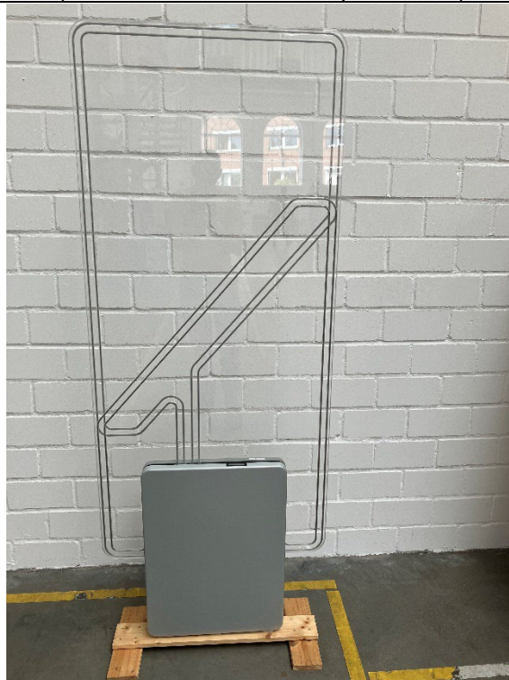
ID ANT1520/700-HPD 2*(1520 mm x 700 mm loop antenna)
