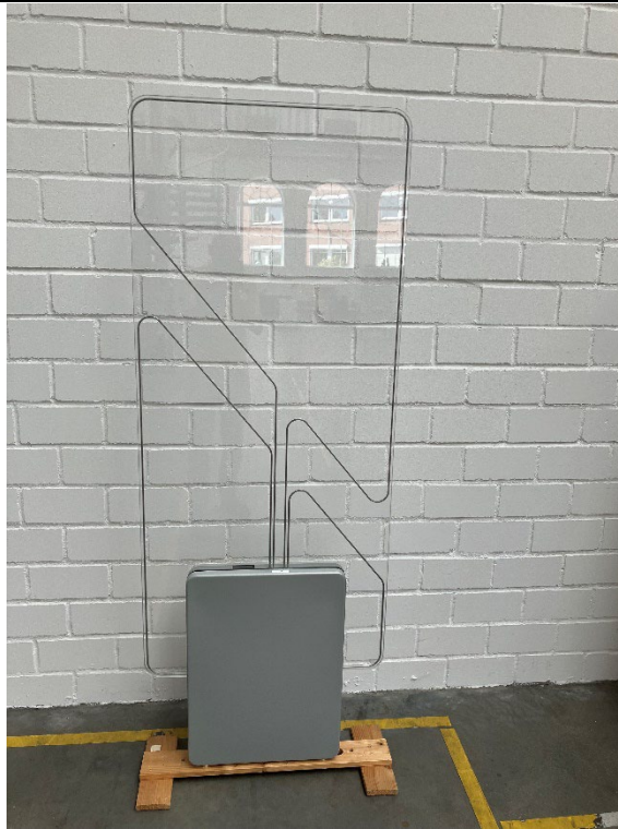
ID ANT1520/680 2*(1520 mm x 680 mm loop antenna)
